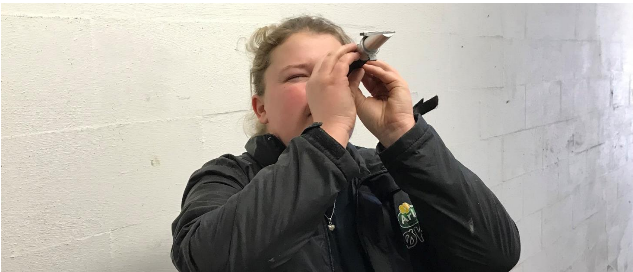
Picture 3: Using a refractometer for testing the antibody concentration in colostrum, is easy to do and is used consistently in the herd, for quality testing and sorting of colostrum
