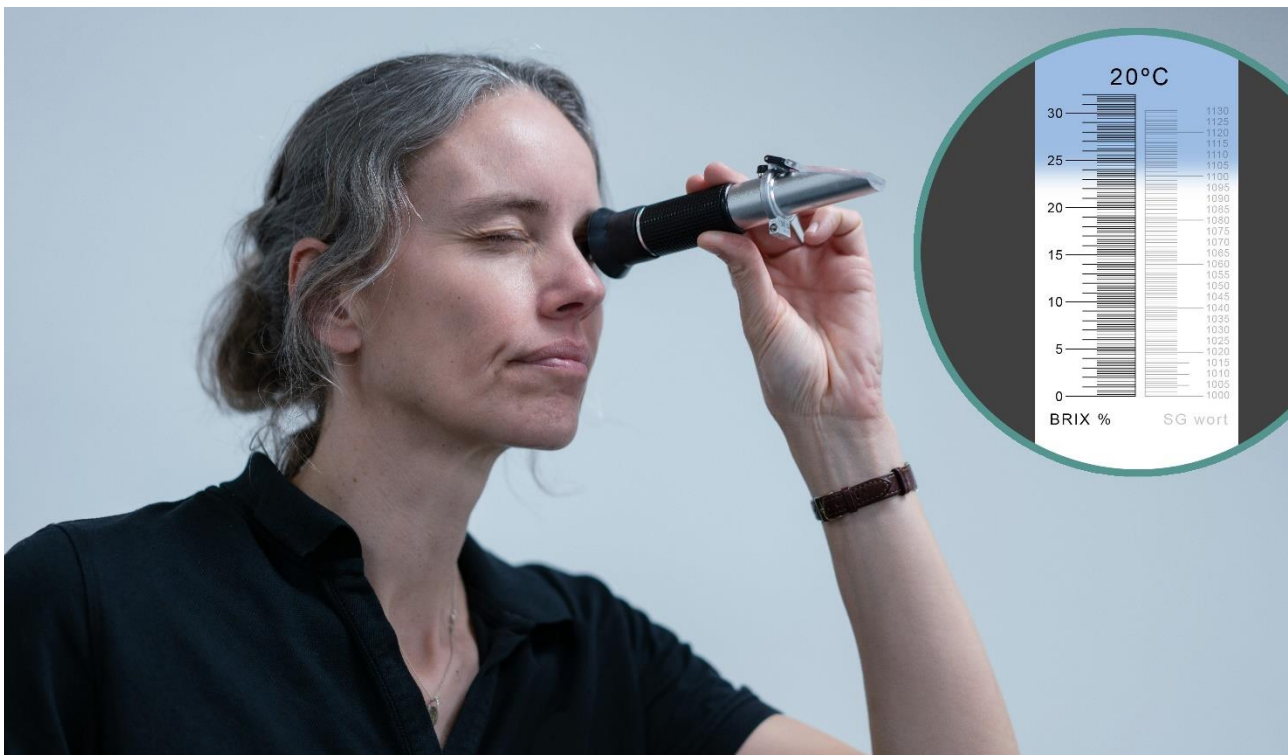
Figure 2: The antibody content of the colostrum should always be tested with a refractometer, with which it is possible to ensure that all calves receive high-quality colostrum.
